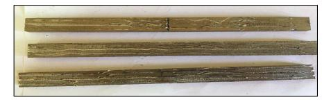
Fig.5C. Bending specimen after ultrasonic peening process
