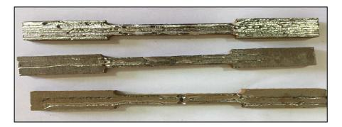
Fig.5B. Tensile sample after ultrasonic peening.
