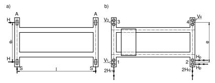
Fig. 1. Ways of imposing a load by cranes a) according to [1], b) according to [2]
