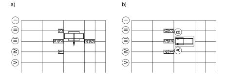
Fig.4. Location of the measuring sensors a) crane's movement, b) braking and hitting into the fenders of the winch
