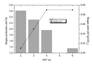
Fig. 4. The relationship between the daily biogas production, biogas yield and hydraulic retention time
