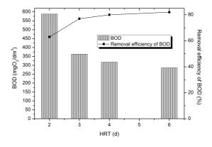
Fig. 3. The influence of the HRT on the degree of BOD removal efficiency and the volume of effluent BOD
