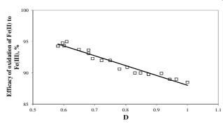
Fig. 2. Effect of coexistence ratio of TOC concentration and concentration of total iron (D) on efficacy in oxidising Fe(II) to Fe(III) (aeration)
