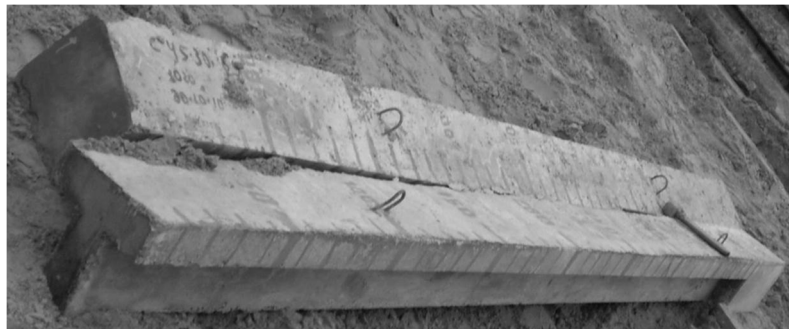
Fig. 2. Specifications of precast concrete T-cross section pile
