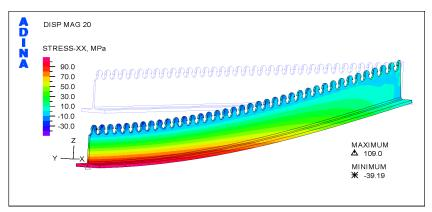
Fig. 9. Normal stress in steel section – view of half length of girder
