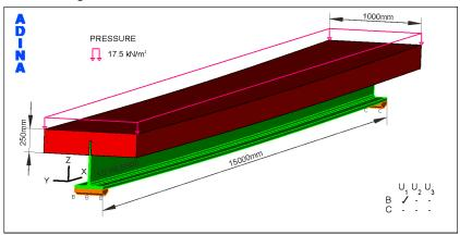
Fig. 7. View of numerical model of girder with assumed load and boundary conditions
