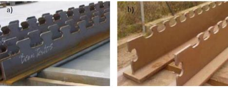
Fig. 3. Shapes of composite dowel shear connections: a) PZ, b) MCL [3]
