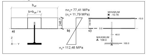
Fig. 12. Distribution of bending stress in connected section: a) computational cross-section of girder, b) distribution of bending stresses determined analytically, c) distribution of stresses in numerical model
