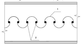
Fig. 4. Shape of web cut: 1 - cutting line, 2 - waste
