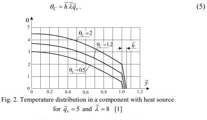
The relation presented above leads to the conclusion that contact temperature increases with the increase in liquid layer's thickness. Temperature distribution
