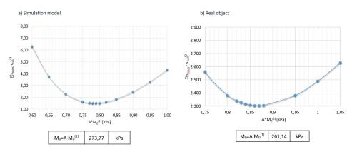
Fig. 8. Results of peat elasticity modulus (constrained modulus) from second method: a) for simulation model; b) for real model
