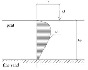
Fig. 2. Stress distribution in the distance l from the force Q by Boussinesq
