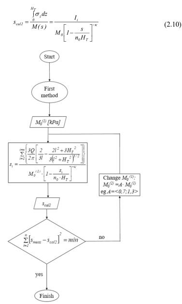
Fig. 3. The calculation algorithm of the second method
