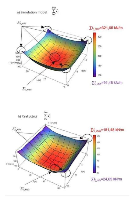
Fig. 6. The stress field from the external load in the peat: a) for simulation model; b) for real model
