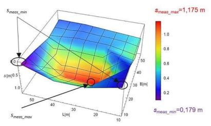
Fig. 5. The measured settlement: a) for simulation model; b) for real model
