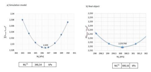
Fig. 7. Results of peat elasticity modulus (constrained modulus) from first method: a) for simulation model; b) for real model
