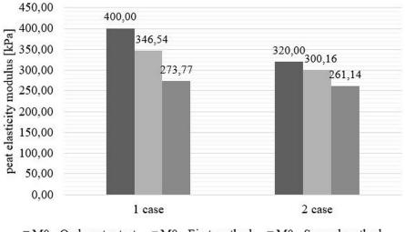
$\blacksquare$  M0 - Oedometer test  $\blacksquare$  M0 - First method  $\blacksquare$  M0 - Second method
