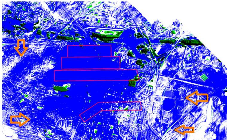
*Fig. 4. Map of falls in the ground level with shading module NDVI, with marked falls deeper than 0,2m in the territory of hard coal mine Centrum between 2010 and 2012, generated in Global Mapper [developed by the author]*
