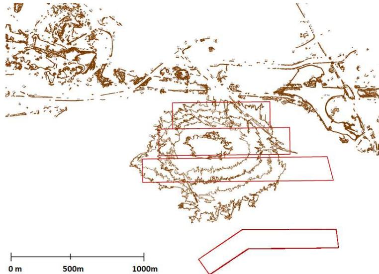
*Fig. 3. Map of isolines of falls in the ground level (subsidence basin) generated in the programme Global Mapper [developed by the author]*
