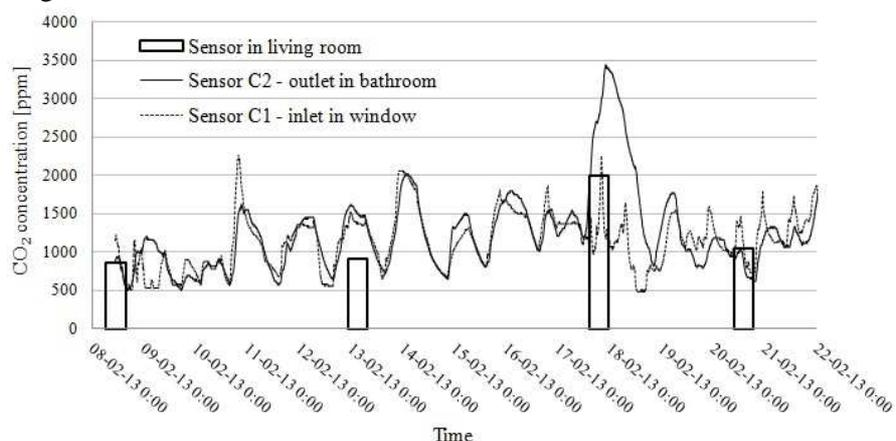
Fig. 10. Variations of CO<sub>2</sub> concentration in the air outlet in the bathroom (sensor C2), in the air inlet in window (sensor C1) and temporary measurements in living room
