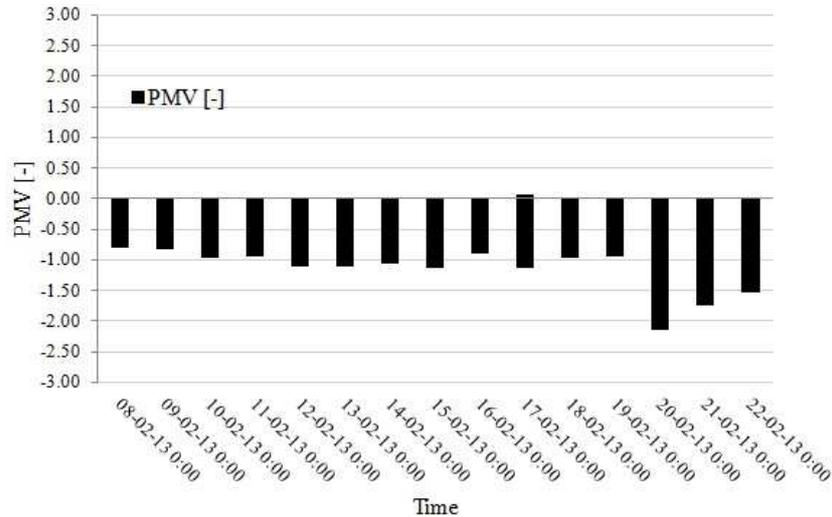
Fig. 13. The average PMV index for test apartment with natural ventilation
