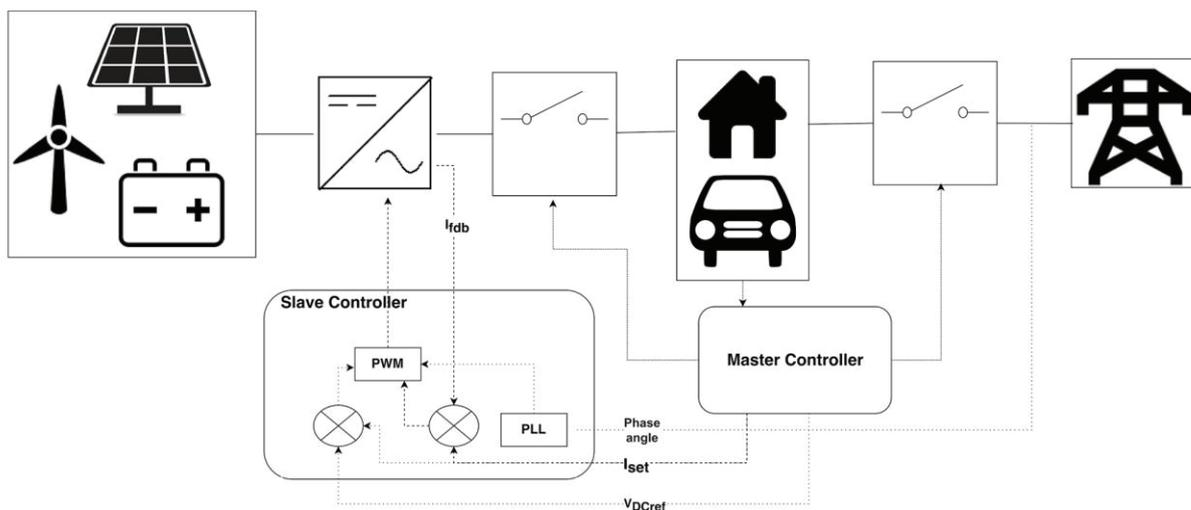
Fig. 1. Diagram of an example Micro Grid
