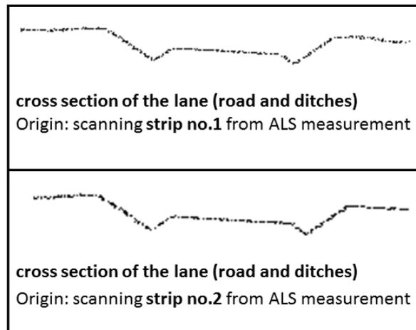
Fig. 7. The sets of points showing a lane, a cross section of the roadway
