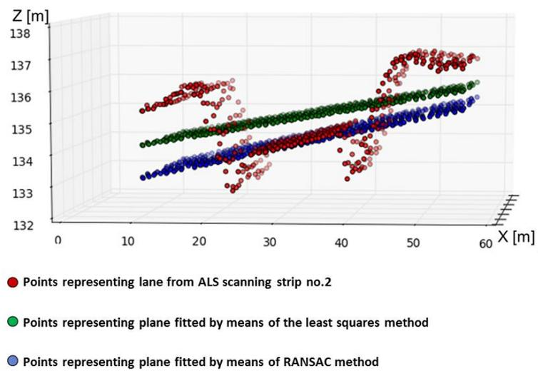
Fig. 9. The plane fitted to the set of points from ALS scanning strip no. 2
