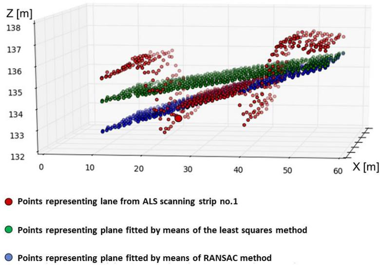
Fig. 8. The plane fitted to the set of points from ALS scanning strip no. 1
