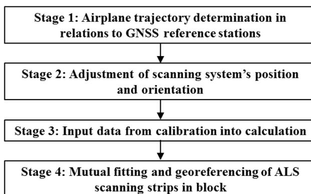
Fig. 2. Process of block adjustment of ALS scanning strips
