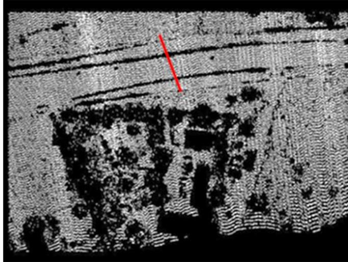
Fig. 6. The fragment of ALS point cloud after filtration, the top view
