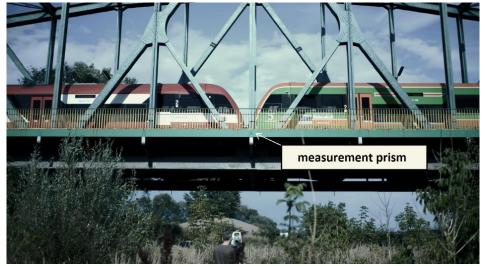
Fig.6. View of the measurement site at the time of crossing by an SA 133 multiple unit [own elaboration]
