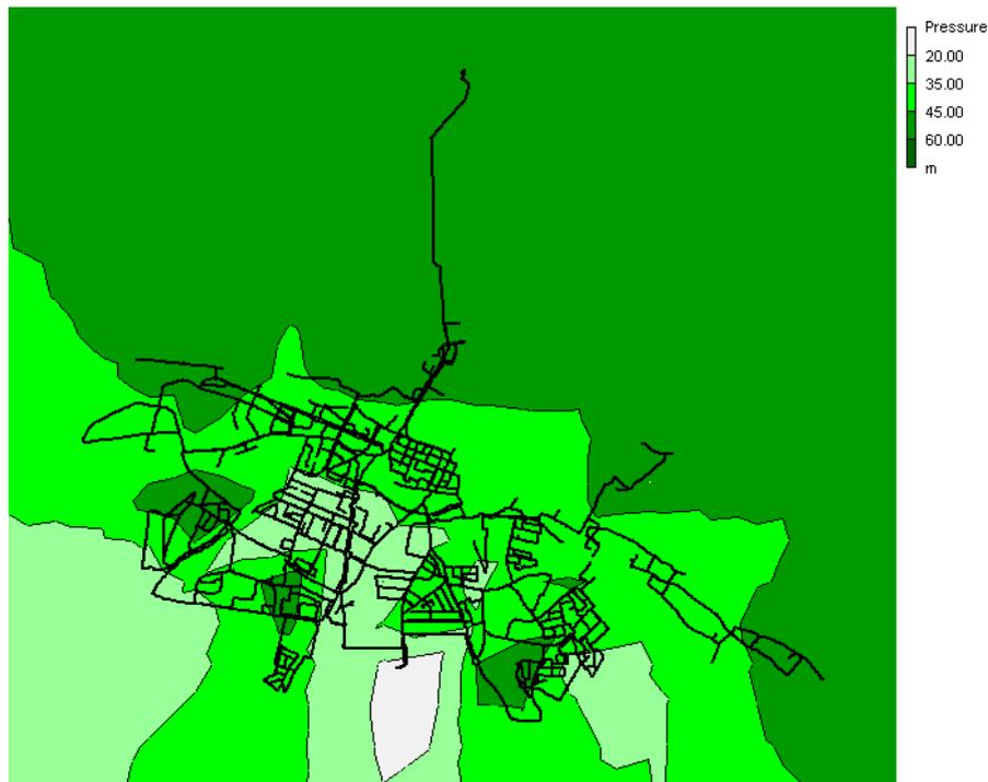
Fig. 5. Contours of water pressure levels in the Głogów system during maximum water consumption
