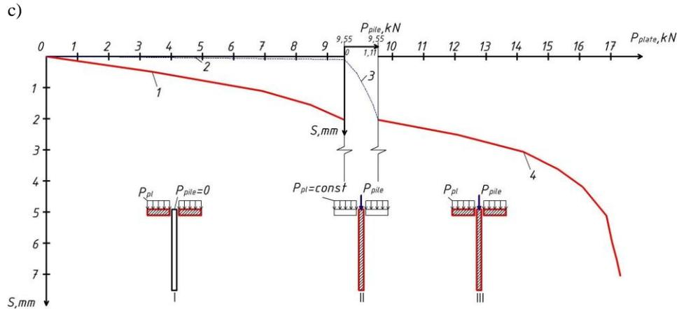
Fig. 7. Graph "Loading- Settlement". III<sup>rd</sup> test of plate segments: 75 mm (a), 125 mm (b), 175 mm (c); 1 – 1<sup>st</sup> stage of plate settlement, 2 – 1<sup>st</sup> stage of pile settlement; 3 – 2<sup>nd</sup> stage of pile loading; 4 – settlement of plate joining a pile
