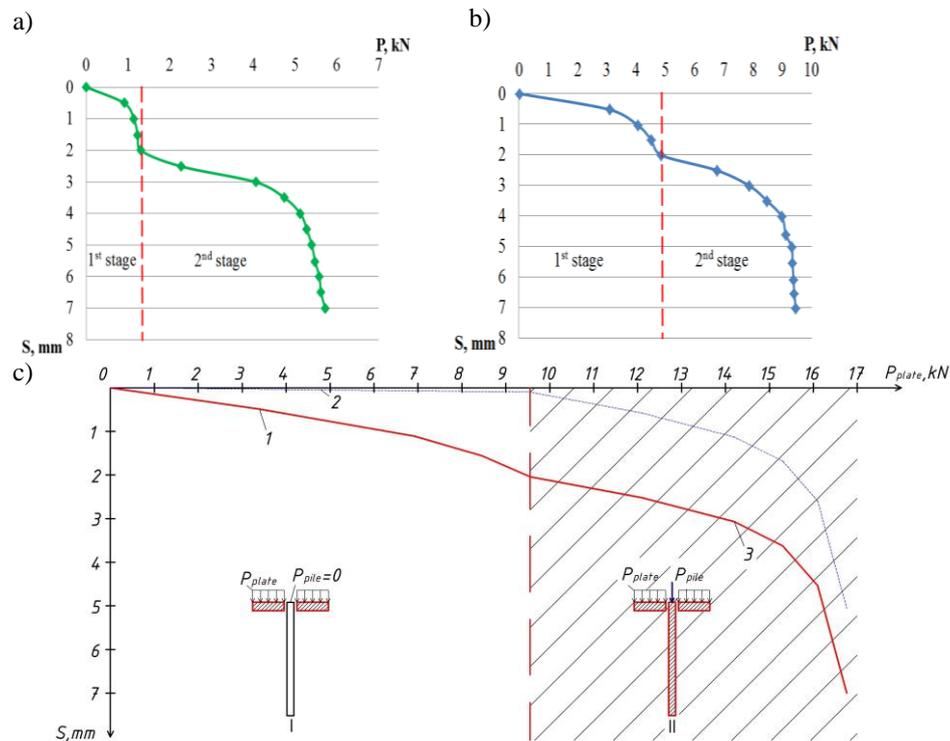
Fig. 6. Graph "Loading– Settlement". II<sup>nd</sup> test of plate segments: 75 mm (a), 125 mm (b), 175 mm (c); 1 – plate settlement, 2 – pile settlement due to additional loading; 3 – settlement of plate joining a pile
