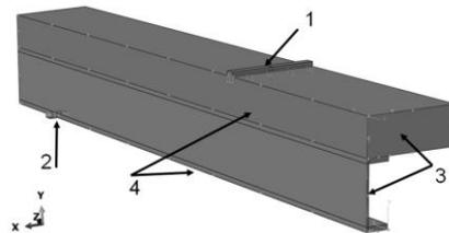
Fig. 5. Boundary conditions: 1 - displacement, 2 - vertical displacement in  $y$  direction (linearly blocked) in the support, 3 - horizontal displacement in  $z$  direction (blocked for the entire cross-section) and rotation around  $x$  and  $y$  axes (blocked), 4 - horizontal displacement in  $x$  direction (blocked for the entire longitudinal section)
