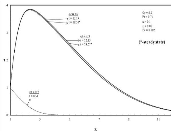
Fig.8. Unsteady outlines of temperature in numerous values of  $\omega t$ .
