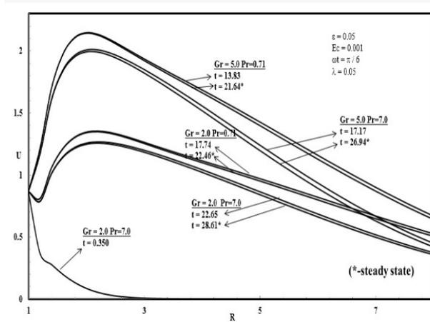
Fig.1. Unsteady outlines of velocity in numerous values of  $Gr$  and  $Pr$ .
