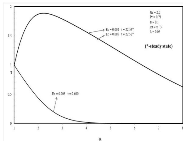
Fig.6. Unsteady outlines of temperature in numerous values of  $Ec$ .
