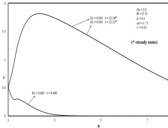
Fig.5. Unsteady outlines of velocity in numerous values of  $Ec$ .
