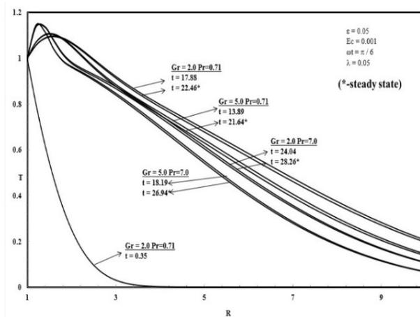
Fig.2. Unsteady outlines of temperature in numerous values of  $Gr$  and  $Pr$ .
