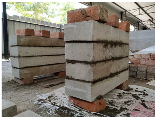
Fig.4. casting of CLC block stack bonded masonry prism
