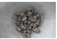
*Phot. 2. Roots mixed with soil clods ground with pestle in a mortar*
