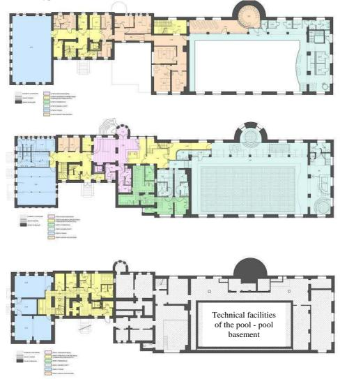
Fig. 1. Plan of the basement, ground and first floors of the building (bottom to top) - the original concept illustrating the distribution of planned functional zones in the facility (based on the conceptual design - from the author's archive)
