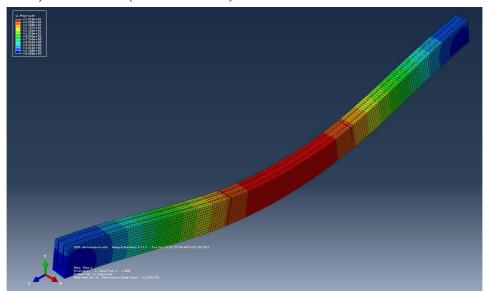
Fig. 3. Distribution of deflections in the beam of solid wood F=30 kN,  $u_{max}$ =18,5 mm
