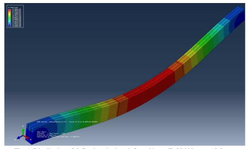
Fig. 4. Distribution of deflections in the reinforced beam F=30 kN,  $u_{\text{max}}\!\!=\!\!12,\!2$  mm
