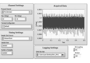
Fig.2. Virtual instrument (VI) written in LabVIEW for verification of PXI-446X device: a - block diagram of the VI, b - front panel of the VI. Results obtained for channel ai3 of PXI-4462 are visible on the graph
