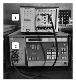
Fig.1. View of the measurement setup: 1 – DC voltage calibrator Fluke 5440, 2 – PXI system with the PXI-6653 (slot 2), PXI-4461 (slot 3), PXI-2567 (slot 4) and the PXI-4462 (slot 5)
