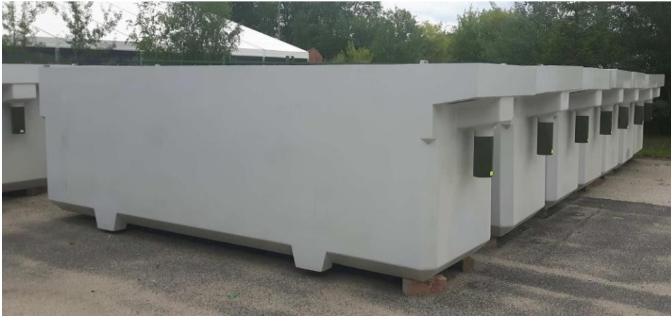
Fig. 1. Newly fabricated electroplating vats
