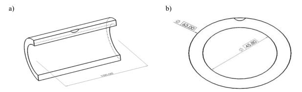
Fig.2. Pipe dimensions and crack orientation: a) transversal crack; b) longitudinal crack.
