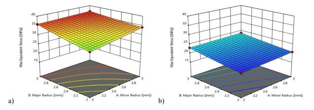
Fig.10. Maximum stress results for the transversal crack a) LCR = 0.25; b) LCR = 0.75.
