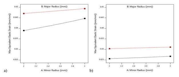
Fig.9. Maximum elastic strain results for the longitudinal crack a) LCR = 0.25; b) LCR = 0.75.
