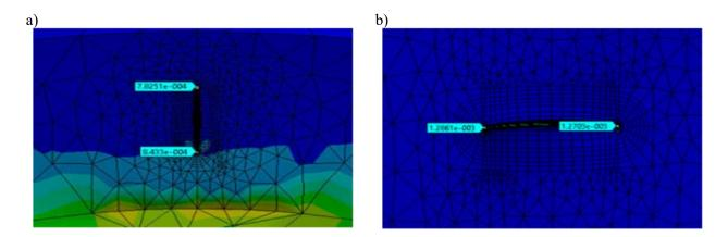
Fig.1. Displacement results: a) longitudinal crack; b) transversal crack [6].
