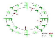
Fig.3. Section view identifying the fixed and pressured faces.
