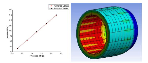
Fig.7. Numerical and analytical von Mises stress results.
