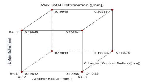
Fig.8. Maximum total displacements for a transversal crack.
