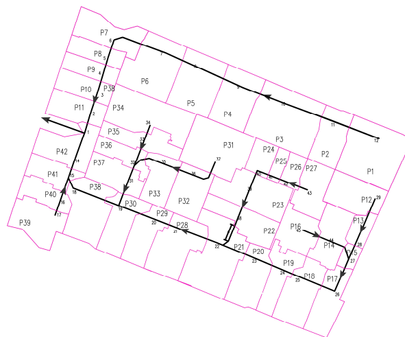
Fig. 2. Diagram of the V catchment - modeled detailed network structure
