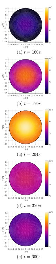
Figure 12: Example of temperature evolution on upper wafer surface (P controller).
