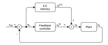
Figure 3: Feedforward ILC scheme
