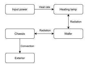
Figure 2: Energy transfer diagram
