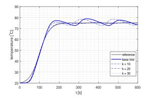
Figure 10: Time responses, PID controller
