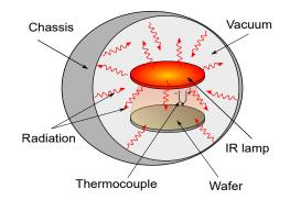
Figure 1: Scheme of vacuum furnace
