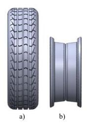
Fig.12. 3D model of a radial tire created using SolidWorks software. a) radial tire; b) rim.
