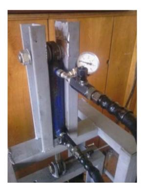
Fig.7. Photo of the manometer, throttles and power cylinder and their place on the rig.
