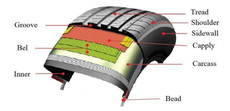
Fig.11. Structure of a radial car tire.
