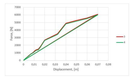
Fig.16. Modification of the deformation of a tire, size 205/55R16: 3 - tire depreciation; 4 - new tire.
