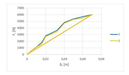
Fig.9. Modification of the deformation of a tire of size 205/55R16. 1 - tire depreciation; 2 - new tire.
