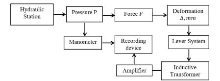
Fig.2. Block diagram for determining car tire elasticity.
