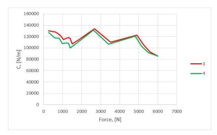
Fig.17. Modification of the deformation of a tire, size 205/55R16: 3 - tire depreciation; 4 - new tire.
