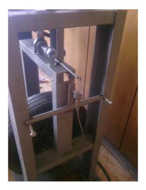
Fig.6. Photo of the lever system and the inductive converter mounted to it.
