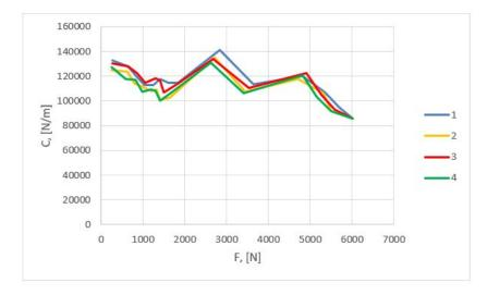
Fig.19. Modification of the elastic constant of a tire of size 205/55R16: 1 - tire depreciation of field experiment; 2 - new tire pattern of field experiments; 3 - tire depreciation of numerical experiment; 4 - new tire pattern of numerical experiment.
