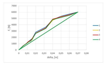
Fig.18. Modification of the deformation of a tire, size 205/55R16: 1 - tire depreciation of field experiment; 2 - new tire pattern of field experiments; 3 - tire depreciation of numerical experiment; 4 - new tire pattern of numerical experiment.
