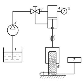
Fig.3. Measurement schematic diagram: 1 - reservoir; 2 - pump; 3 - regulator; 4 - cylinder; 5 - manometer; 6 - pneumatic tire; 7 - measuring device.
