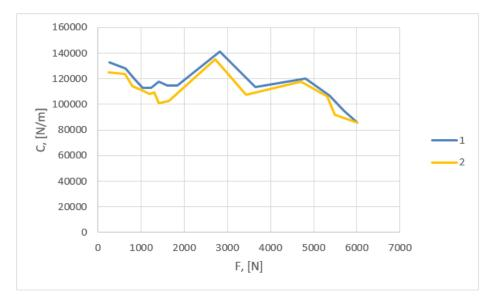
Fig.10. Modification of the elastic constant of a tire, size 205/55R16. 1 - depreciated tire; 2- new tire.
