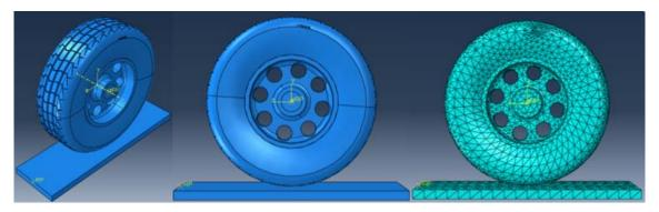
Fig.13. Three-dimensional FEM model of tire in Abaqus environment.
