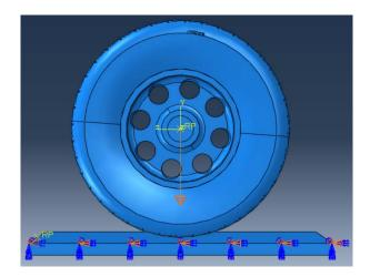
Fig.14. Application of external loads.
