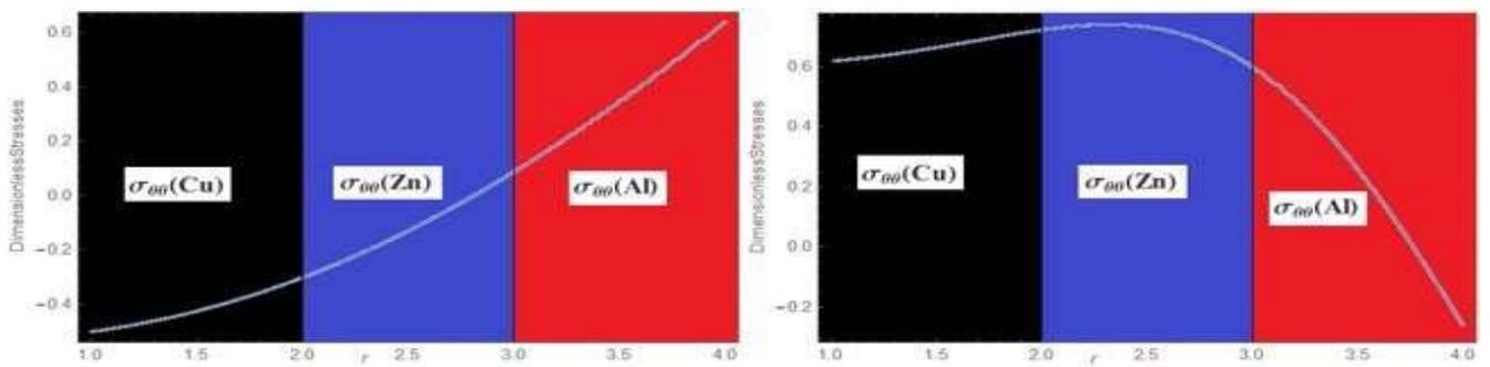
Fig.6(c). Plot of  $\sigma_{\theta\theta}$  along  $r$ .
