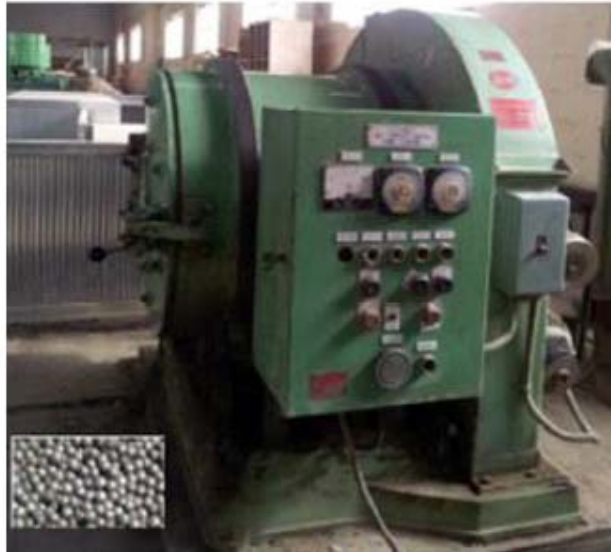
Fig.3. Shot peening machine with shot balls.
