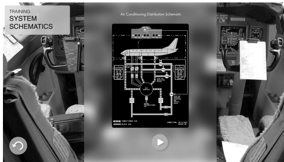
Fig. 10. Second level FSM output as a schematic of the AC distribution in an aircraft.
