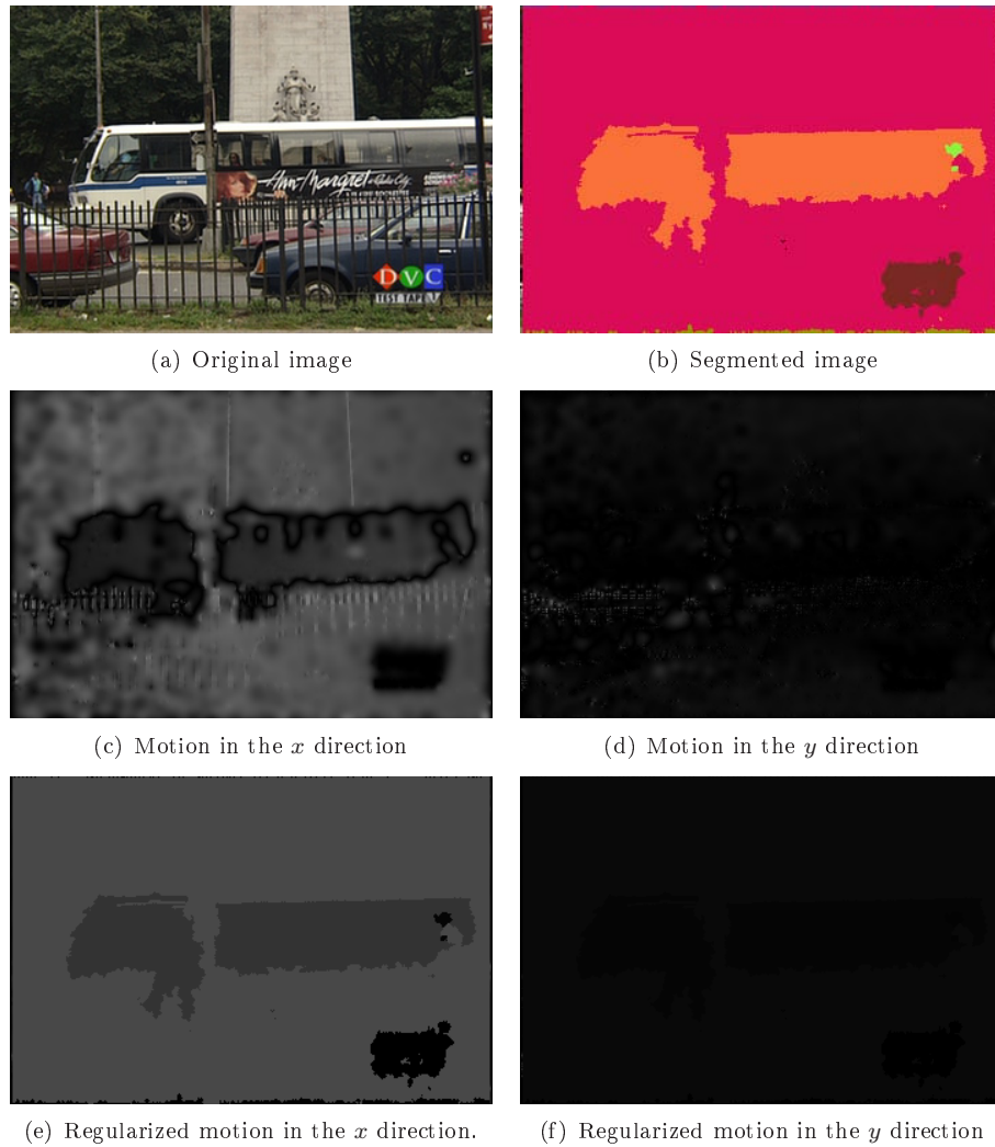
Fig. 6.6. Frame 112 from the ‘Bus’ sequence segmented using multi-label fast marching
