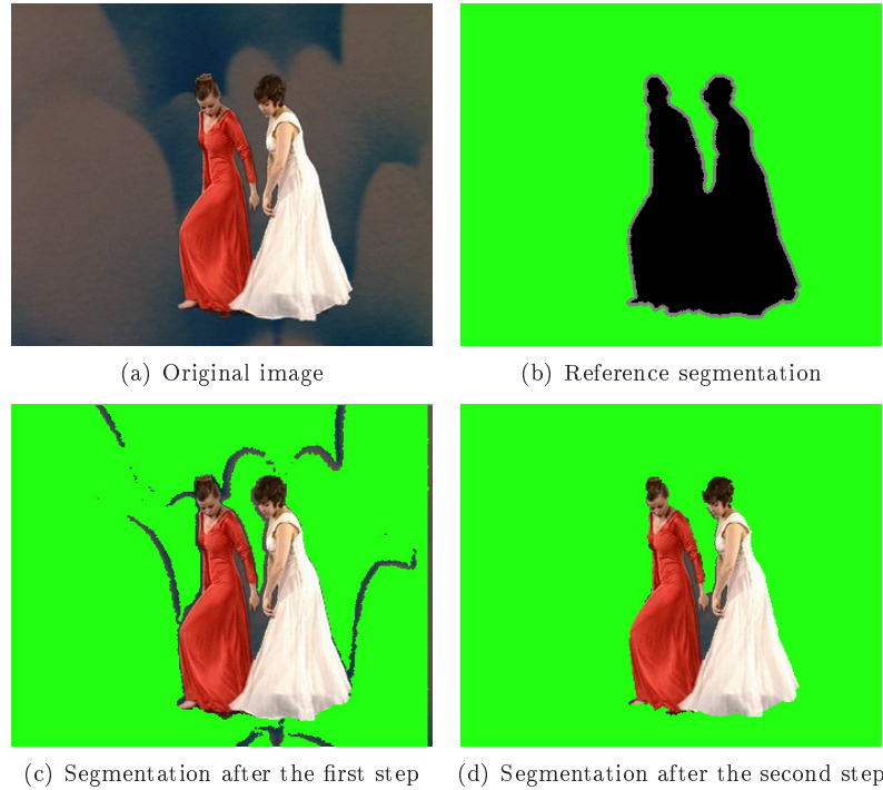
Fig. 5.16. Frame 47 from the ‘Dance’ sequence segmented using two-step fast marching
