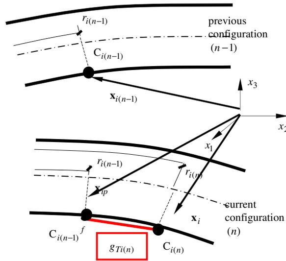
Fig. 2. A tangential gap increment
