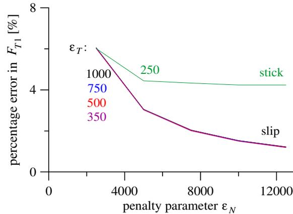
Fig. 14. Example 3 – tangential contact force
