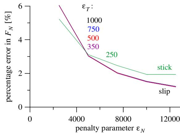
Fig. 13. Example 3 – normal contact force
