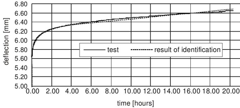
Fig. 5. Identification of rheological parameters of the material
