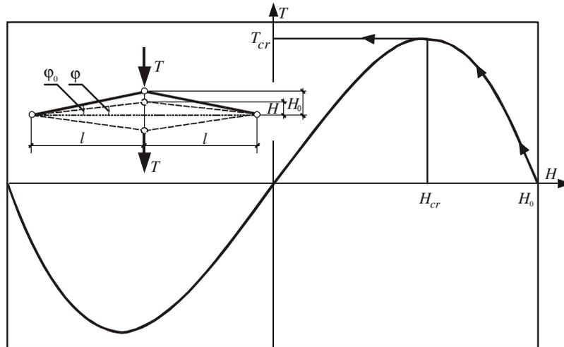
Fig. 3. The elastic solution of the Mises truss
