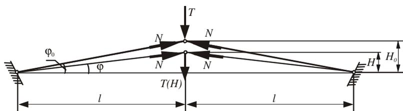
Fig. 2. The Mises truss
