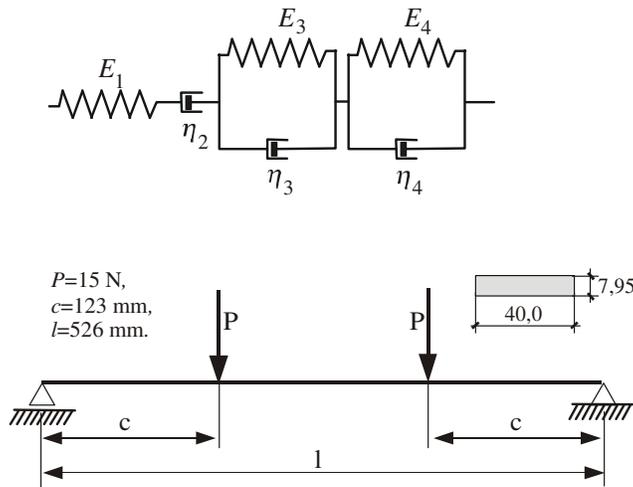
Fig. 4. The six parameter mechanical model of the material and the static scheme for the creep bending test
