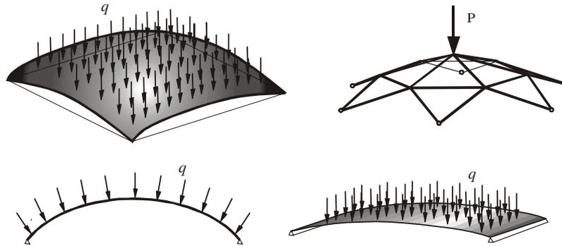
Fig. 1. Shallow space trusses, arches and shells
