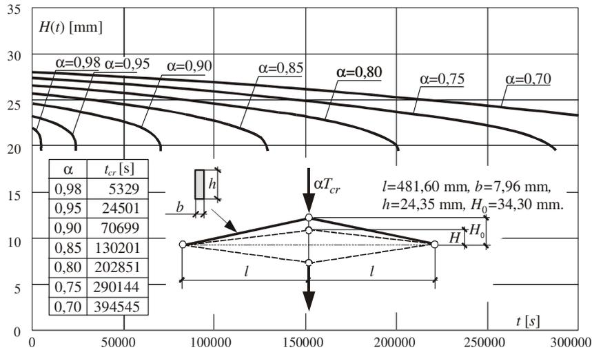
Fig. 6. Stability of the viscoelastic Mises truss
