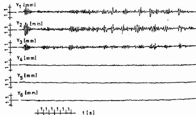
Fig.5. Results of loading bay No. 5 with the winch hitting the fenders 1,2,3,4,5,6 – numbers of measuring sensors
