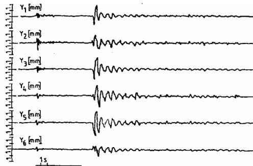
Fig.6. Results of imposing a load on bay No.1 caused by the movement of a loaded crane
