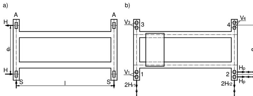
Fig. 1. Ways of imposing a load by cranes
