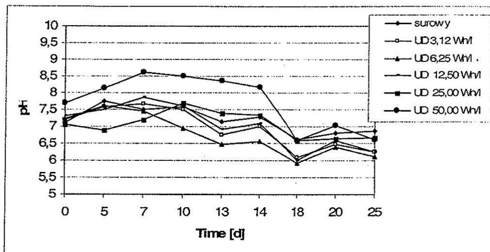
Fig. 6. pH changes during aerobic stabilization
