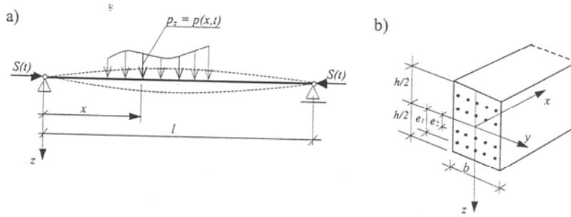
Fig. 2 Simply supported beam loaded by transverse load  $p(x, t)$  and by axial load  $S(t)$ : a) model b) example of the symmetric reinforcement of the cross section with two pair of long fibre families.
