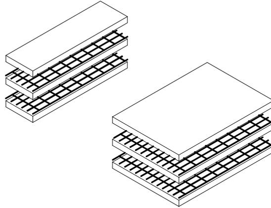
Fig. 1 Construction element reinforced with the layers of long fibres.
