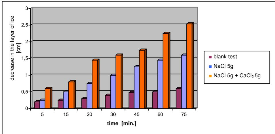
Fig. 8. The impact of NaCl and the mixture of NaCl + CaCl<sub>2</sub> on the effectiveness of ice melting
