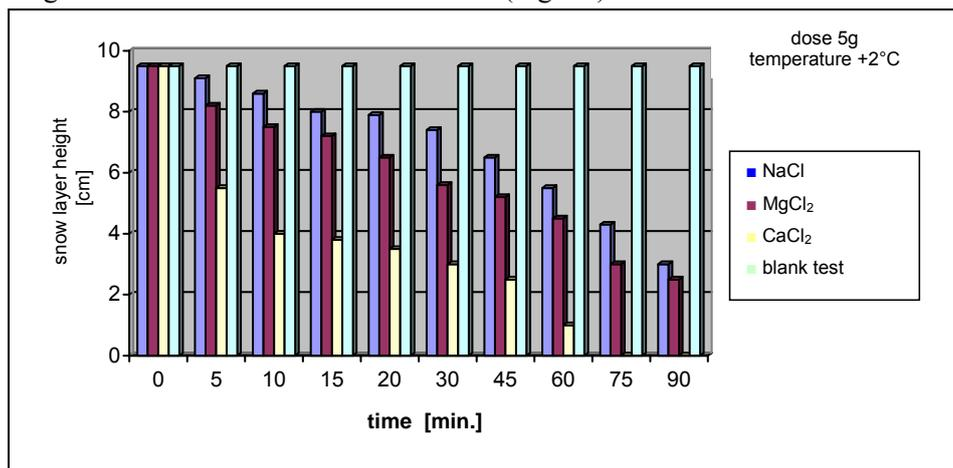
Fig. 12. The efficiency of activity of chemical compounds used in the dose of 5g in the temperature of +2 °C
