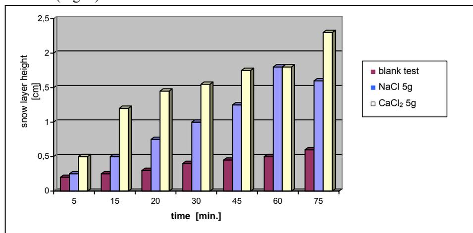
Fig. 1. The impact of NaCl and CaCl<sub>2</sub> on the effectiveness of snow melting
