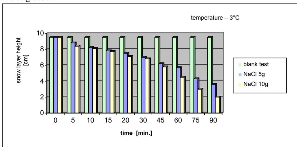
Fig. 2. The impact of NaCl on the effectiveness of snow melting in the temperature of  $-3^{\circ}\text{C}$
