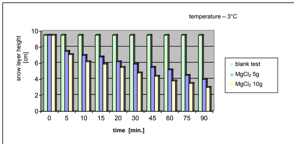
Fig. 10. The impact of MgCl<sub>2</sub> on the efficiency of snow melting in the temperature of -3°C
