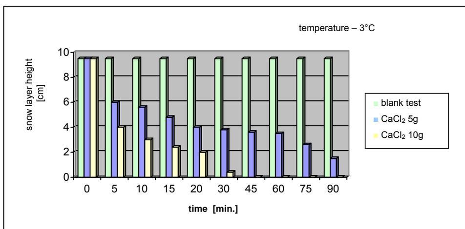
Fig. 3. The impact of  $\text{CaCl}_2$  on the efficiency of snow melting in the temperature of  $-3^{\circ}\text{C}$
