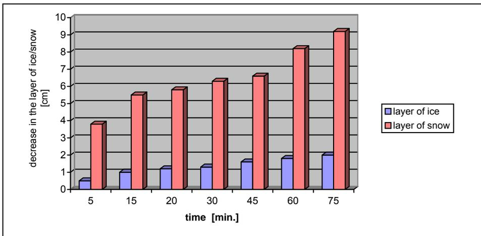
Fig. 5. The comparison of activity of CaCl<sub>2</sub> (the dose of 5g) on the effectiveness of snow and ice melting
