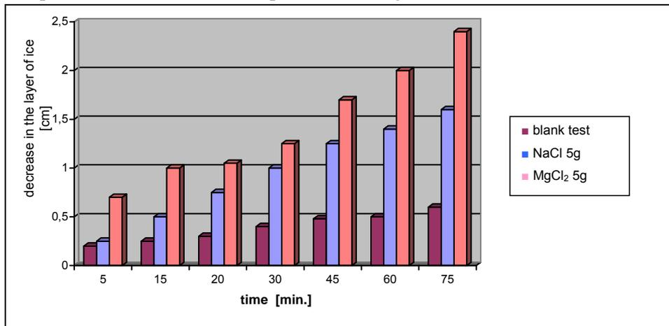
Fig. 9. The impact of NaCl + MgCl<sub>2</sub> on the efficiency of ice melting
