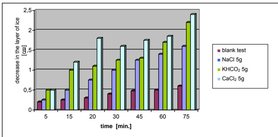
Fig. 7. The impact of  $\text{NaCl}$ ,  $\text{KHCO}_2$  and  $\text{CaCl}_2$  on the efficiency of ice melting
