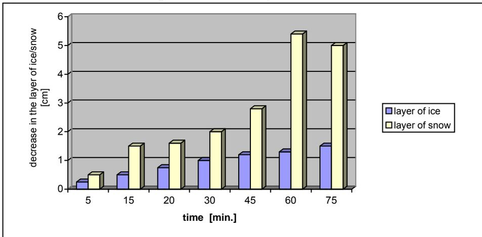
Fig. 4. The comparison of activity of NaCl (in the dose of 5g) on the effectiveness of snow and ice melting
