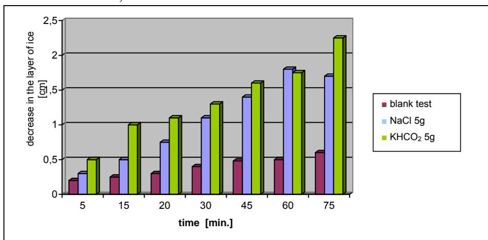
Fig. 6. The impact of  $\text{NaCl}$  and  $\text{KHCO}_2$  on the effectiveness of ice melting
