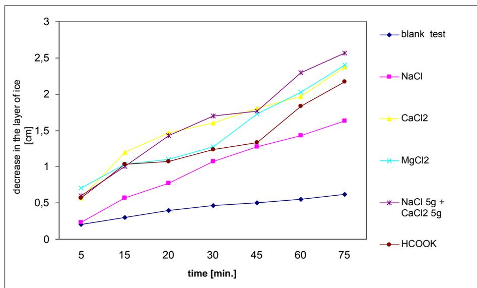
Fig. 11. A collective comparison of the impact of chemical agents on the speed of ice melting
