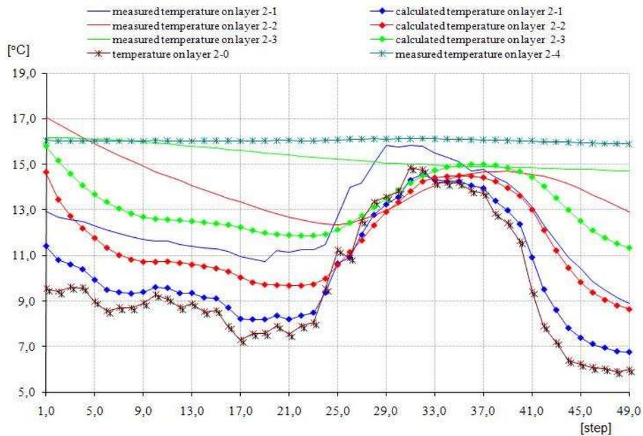
Fig 6. The temperature distribution registered on 17.05.2007 for the road pavement construction with crusher-run base course
