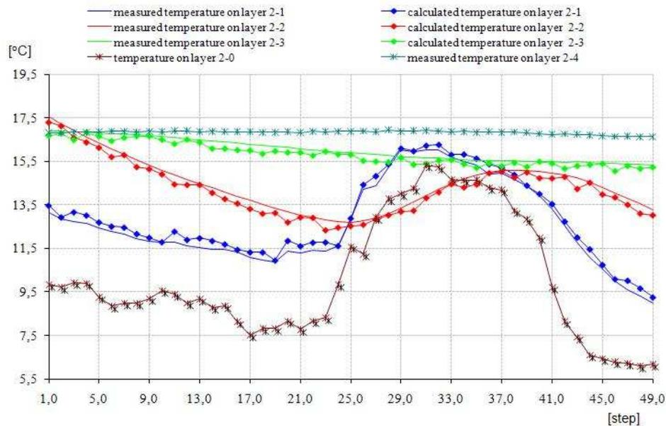
Fig 7. The temperature distribution registered on 17.05.2007 for the road pavement construction with crusher-run base course
