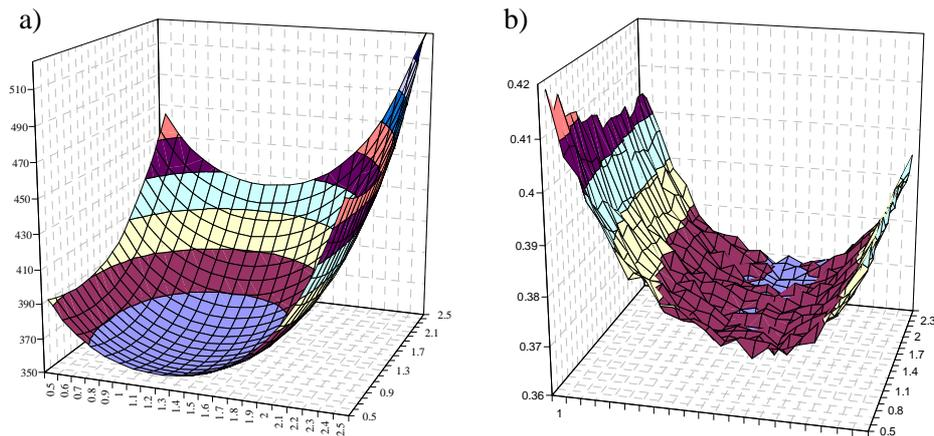
Fig 8. The criterion surfaces  $\varphi(\mathbf{v})$  for the vector  $\mathbf{v} = (\lambda_1, \lambda_2)$  of coefficients of thermal conductivity: a) the criterion of least squares, b) the criterion of minimax
