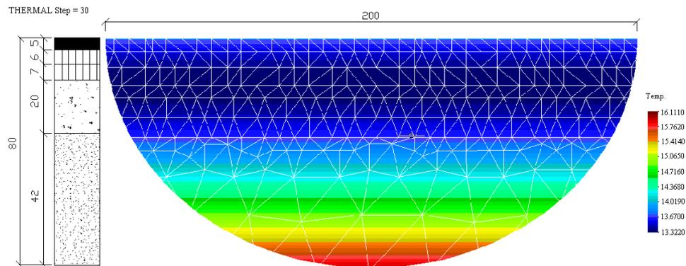
Fig 4. Temperature distribution at the 24-th hour of the analysis
