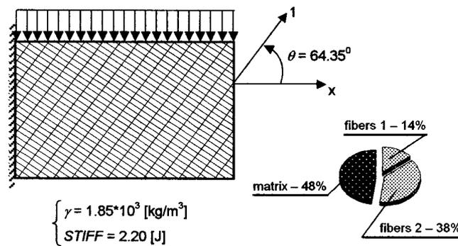
Fig. 8. Optimal disk reinforced with fiber mat – case 2
