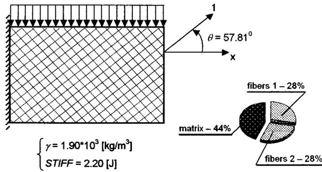
Fig. 7. Optimal disk reinforced with fiber mat – case 1
