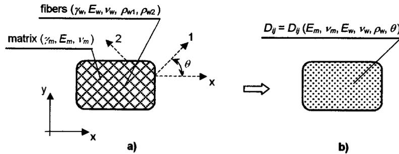
Fig. 2. Material reinforced with fiber-mat: a) real composite, b) model of composite
