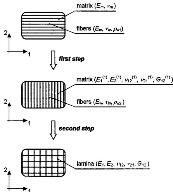
Fig. 3. Two steps of modeling process for material reinforced with fiber-mat
