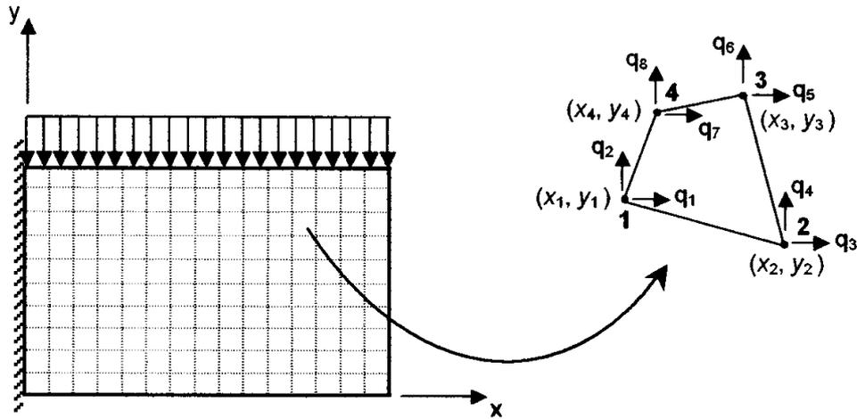
Fig. 6. Discretization of disk domain using finite elements
