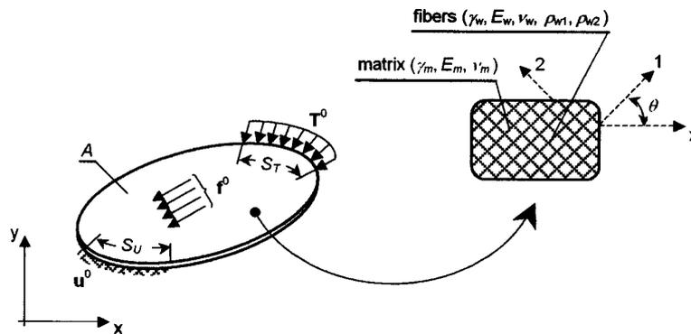
Fig. 1. Two-dimensional composite disk subjected to service loading
