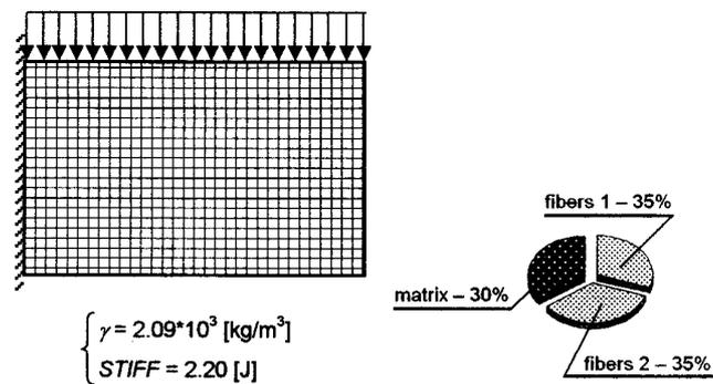
Fig. 9. Reference disk reinforced with fiber mat
