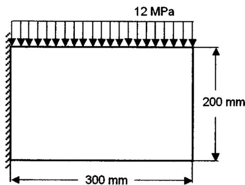
Fig. 5. Composite disk subjected to load and boundary conditions
