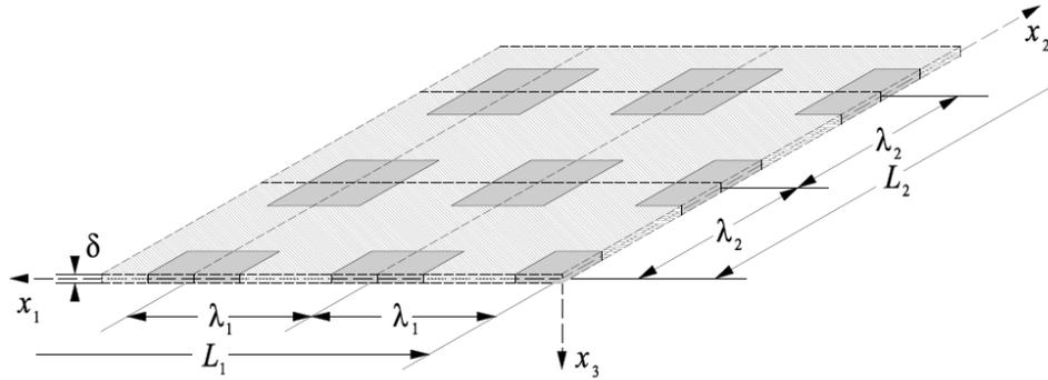
Fig. 1. A fragment of a thin periodic plate
