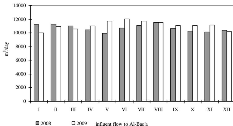
Fig.3. Influent flow of raw wastewater to Al-Baq'a WWTP in 2008/2009
