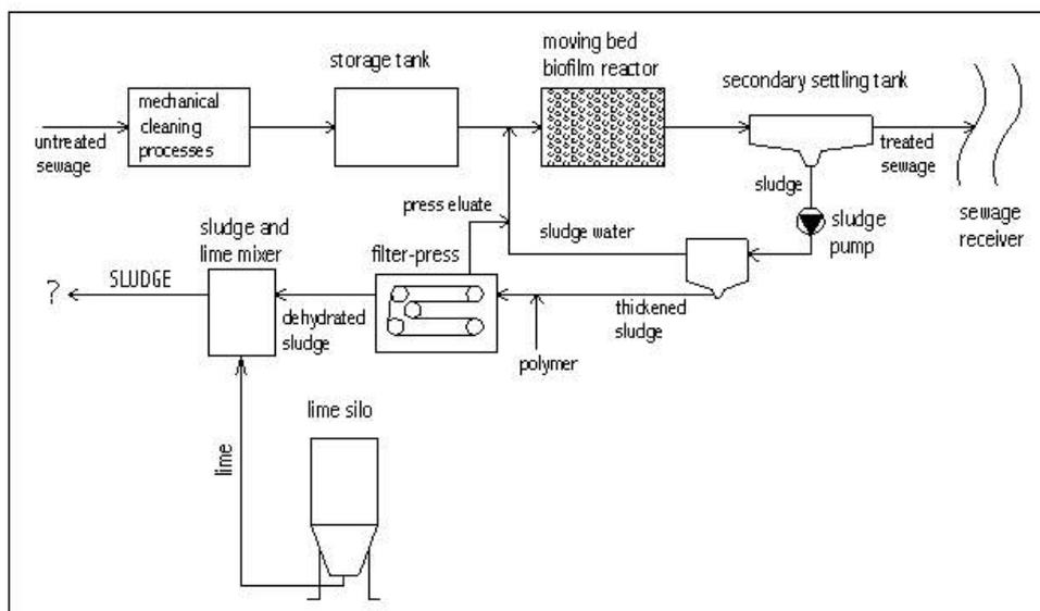
Figure 1. The flow chart of sewage treatment plant
