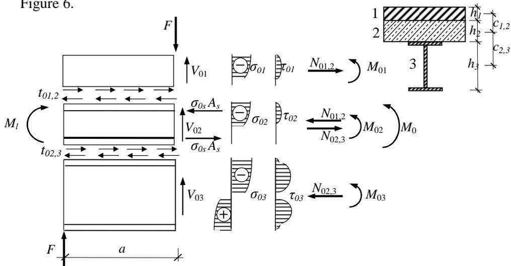
Fig. 6. Forces and stresses in the three-layer beam in the state of load carrying capacity with slip
