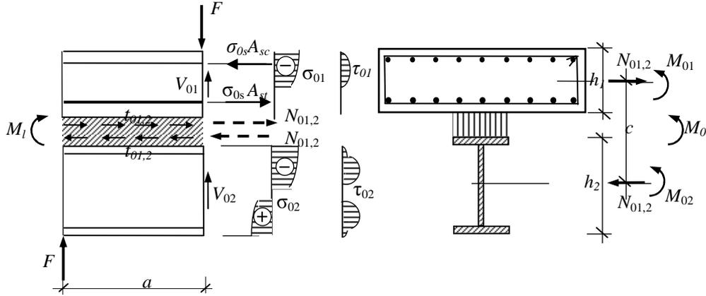
Fig.3. Forces and stresses in the reinforced concrete-steel beam in the limit state of load carrying capacity with slip
