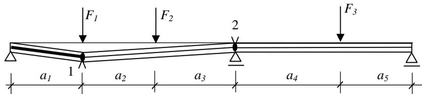
Fig.1. Two-layer reinforced concrete-steel beam in the limit state with slip
