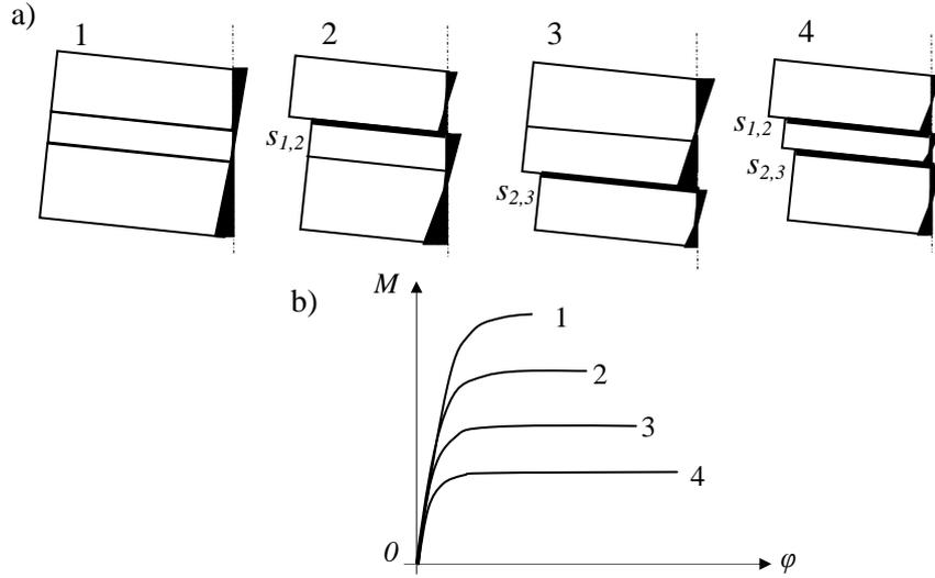
Fig. 7. Three-layer beam, a) destruction mechanisms 1...4; b) relationship moment  $M$  vs angle  $\varphi$  for mechanisms 1...4
