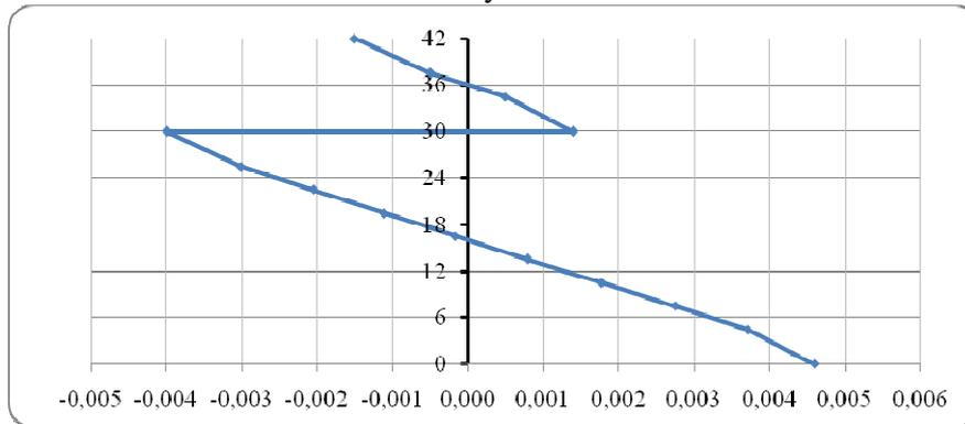
Fig. 17. Strains in section  $\beta$ - $\beta$  of two-layer beam with slip
