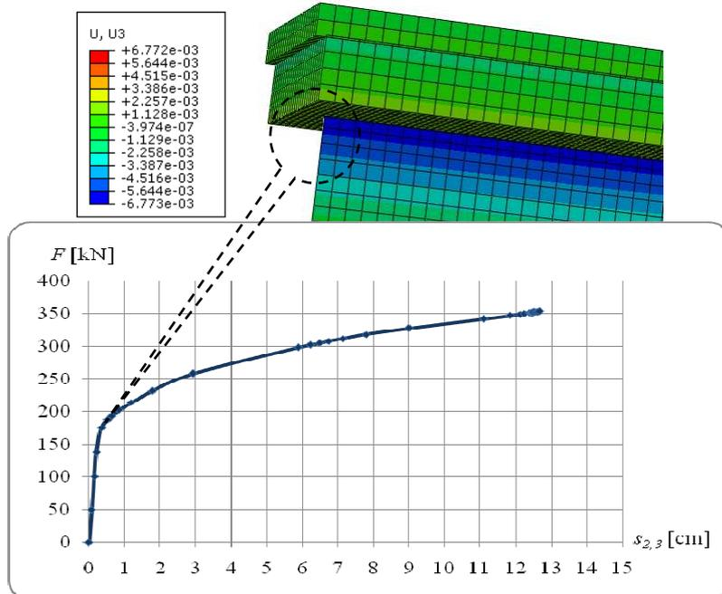
Fig. 14. The relationship of slip  $s_{2,3}$  vs loading force  $F$  in three-layer beam
