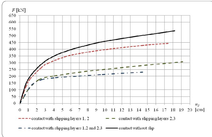
Fig. 12. The relationship of load  $F$  vs the vertical displacement  $u_2$  in the middle of the span of three-layer composite beam
