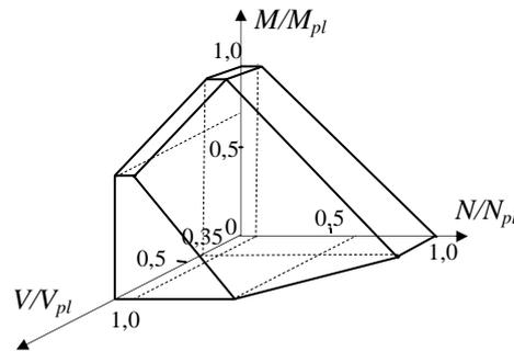
Fig. 5. Limit surface for  $M - N - V$  of steel I-beam cross section by PN-EN 1993-1-1
