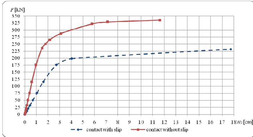
Fig. 11. The relationship of load  $F$  vs the vertical displacement  $u_2$  in the middle of the span of two-layer composite beam
