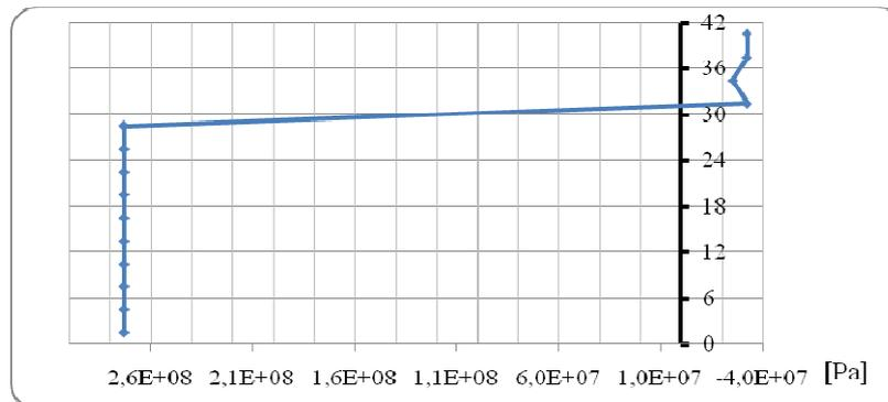
Fig. 15. Von Mises stresses  $\sigma_{red}$  in section  $\alpha$ - $\alpha$  of two-layer beam without slip
