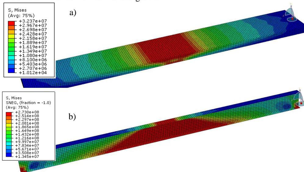
Fig. 16. The fields of stresses  $\sigma_{red}$  for two-layer beam without slip: a) in the plate, b) in the steel beam
