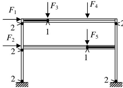
Fig. 9. Mechanism of the destruction for the composite frame, taking into account slip
