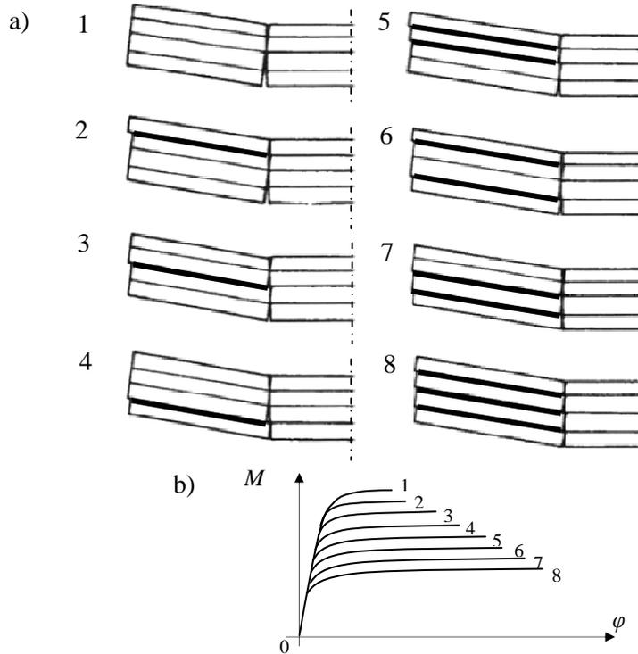
Fig. 8. Four-layer beam, a) destruction mechanisms 1...8; b) relationship moment  $M$  vs angle  $\varphi$  for mechanisms 1...8
