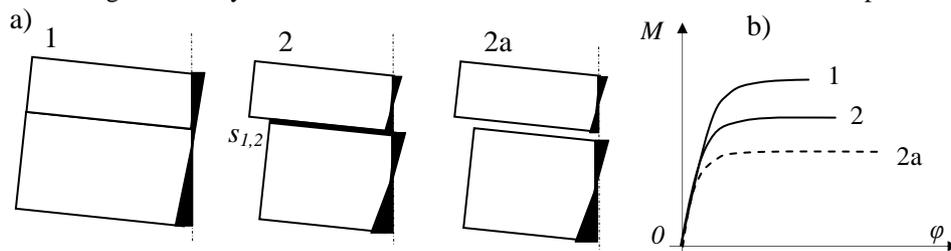
Fig. 2. Two-layer beam, a) destruction mechanisms 1...2a; b) relationship moment  $M$  vs angle  $\varphi$  for mechanisms 1...2a
