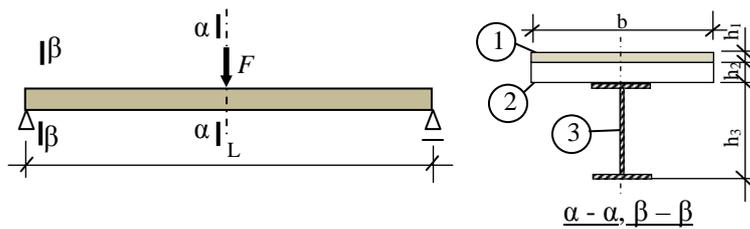
Fig. 10. Scheme with loading and cross-section of composite beam
