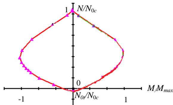
Fig. 4. Function of strength  $\varphi(M, N)$  for the reinforced concrete layer
