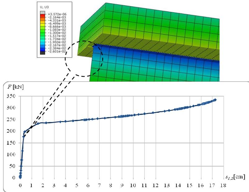
Fig. 13. The relationship of slip  $s_{1,2}$  vs vertical force  $F$  in two-layer beam
