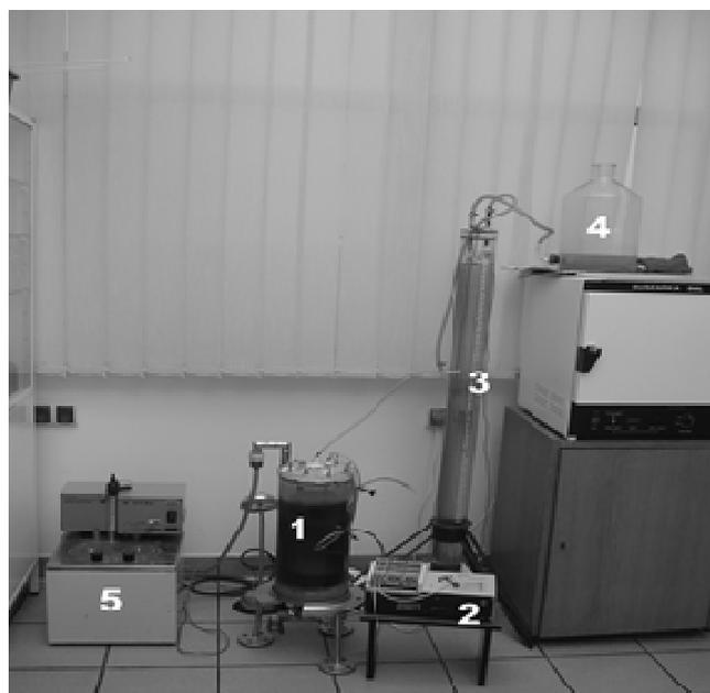
1. UASB bioreactor
