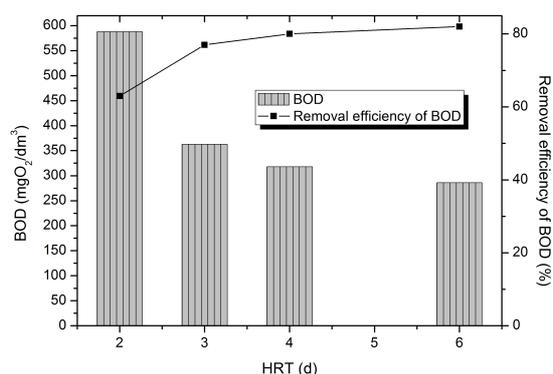
Fig. 3. The influence of the HRT on the degree of BOD removal efficiency and the volume of effluent BOD
