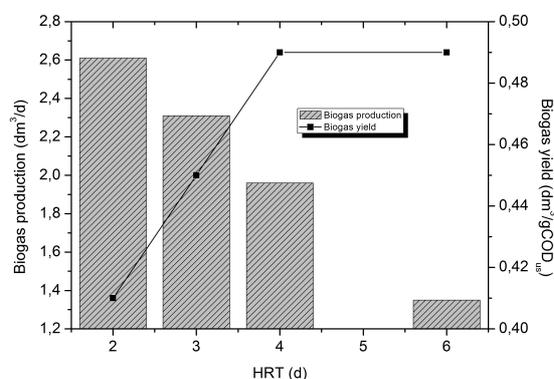
Fig. 4. The relationship between the daily biogas production, biogas yield and hydraulic retention time
