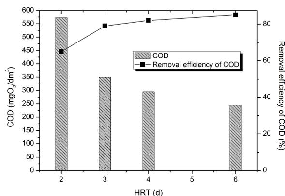
Fig. 2. The influence of the HRT on the degree of COD removal efficiency and the volume of effluent COD
