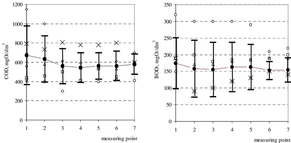
Fig. 5. Changes in COD and BOD<sub>5</sub> in the sewage at measuring points (5 series) and standard deviation of average values
