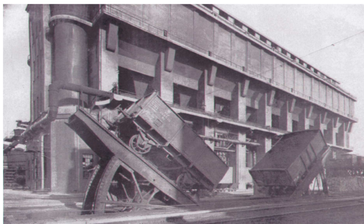
Fig. 6. Wagon discharger, view at the south wall of the the Koppers' boiler room building
