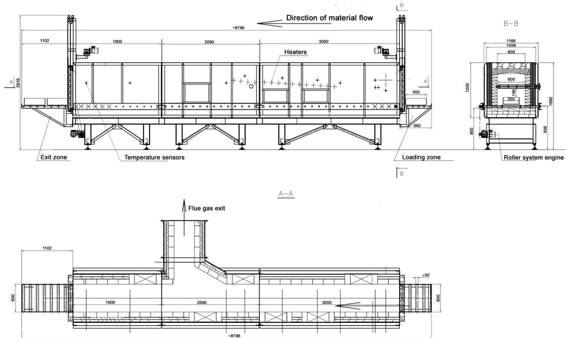
Fig. 2. Scheme of the tannery waste incinerating installation
