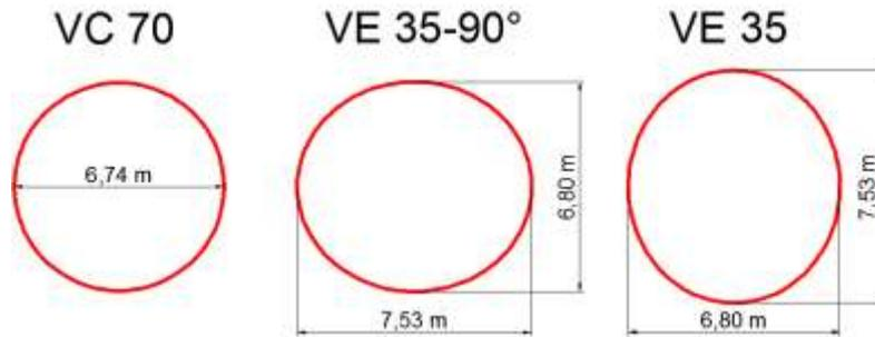
Fig. 8. Shapes and general dimensions of compared shells
