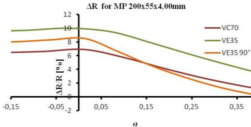
Diagram 7. Change of the radius of curvature depending on backfill height for a shell of 4,00 mm thickness
