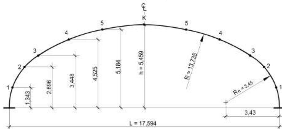
Fig. 5. Locations of the measurement points and shell geometry
