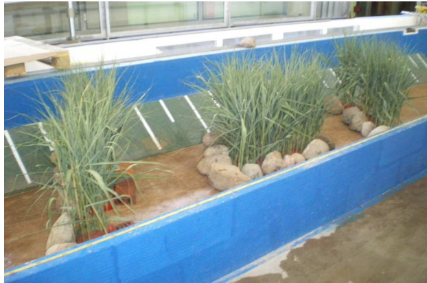
Fig. 6. Laboratory model of fishway with biotechnical build-up
