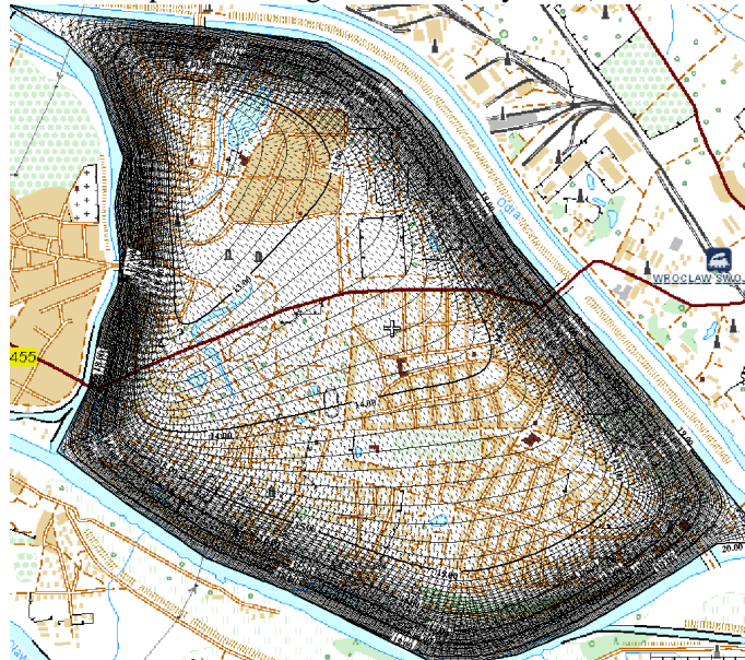
Fig. 11. Hydroisohips and velocity field of 12 July, 1997
