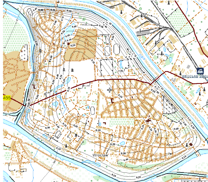
Fig. 16. Hydroisohips and velocity field of 12 October, 1997
