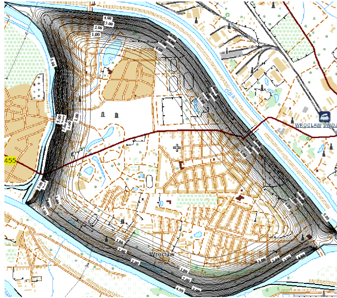
Fig. 12. Rise of groundwater level of 12 July, 1997
